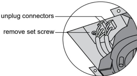
10.) Remove the electrical cover set screw and slide open the electrical enclosure. Connect wiring using the provided QUICK CONNECTS (U.S.A.) or WIRE NUTS (Canada).
