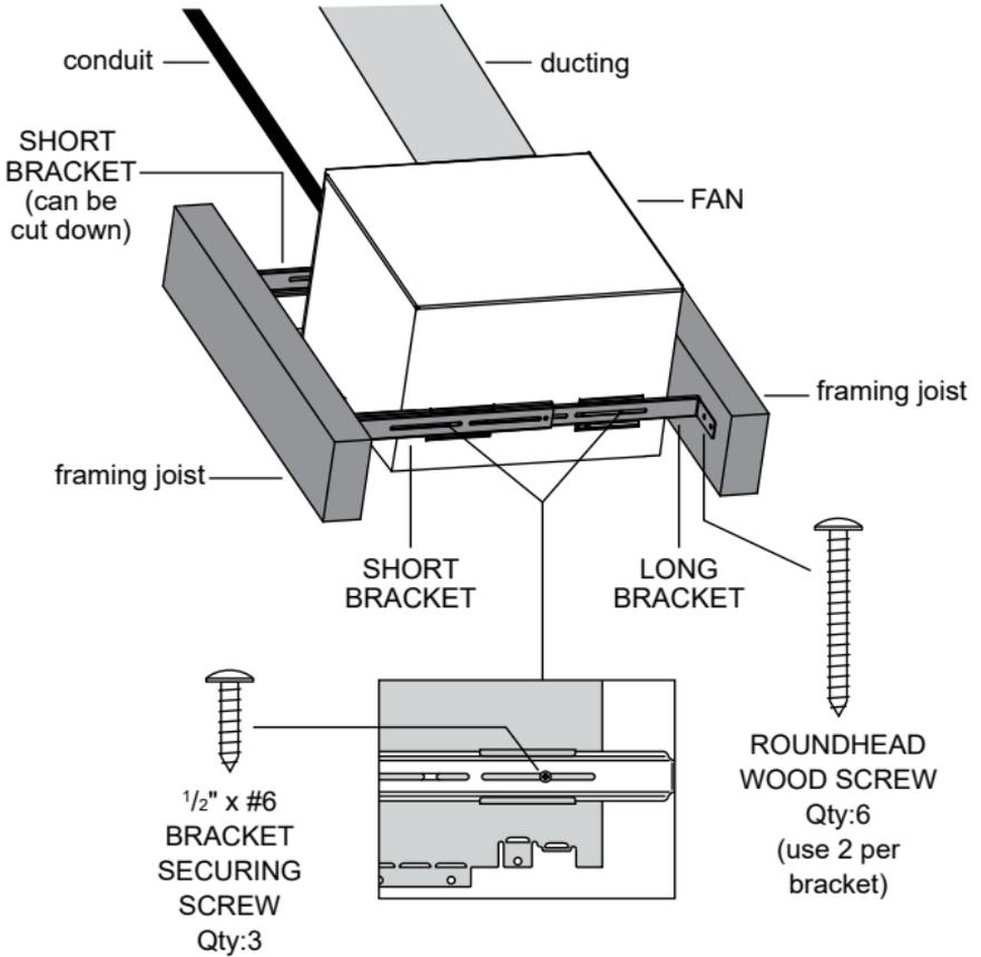
4.) Attach conduit with wiring to FAN.
