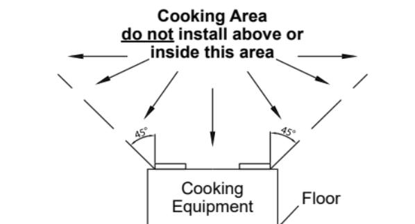
Do not install ventilation fan in areas where the duct work will require configuration as shown.
