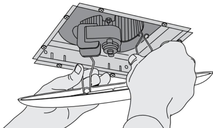
3.) Your existing fan may be attached in several ways. Look for attachment screws in the ceiling and remove. Your fan may also be attached on the attic side, which will require you to access it from the attic. Locate attic attachment screws and remove.
