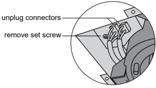
7.) Remove the electrical cover set screw and slide open the electrical enclosure. Connect wiring using the provided QUICK CONNECTS (U.S.A.) or WIRE NUTS (Canada).
