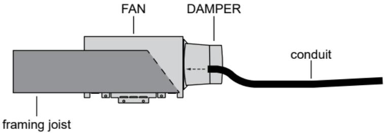
5.) Attach DAMPER to ducting.
