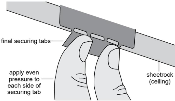
13.) Align TRIM RING notch to vent (DAMPER) position. Attach TRIM RING to FAN. TRIM RING attaches to FAN body and clicks into place when secure.
