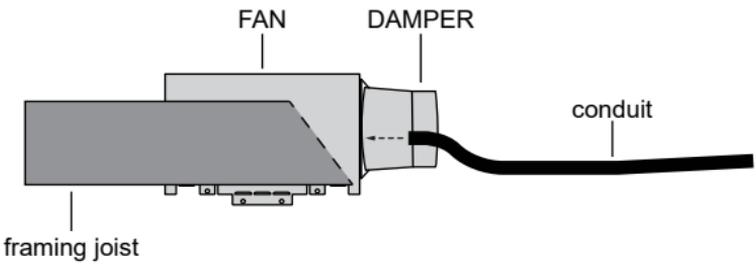
5.) Attach DAMPER to ducting.
