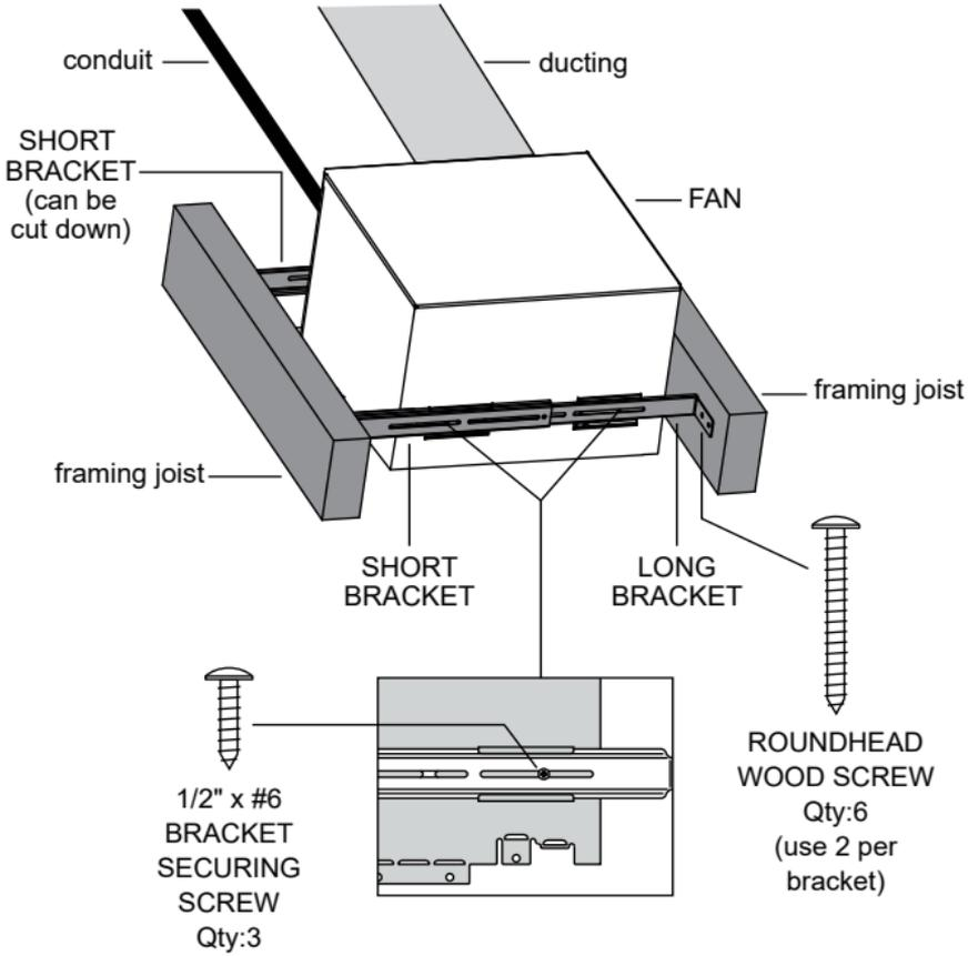
4.) Attach conduit with wiring to FAN.
