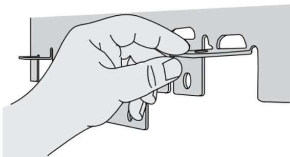
3.) Attach FAN to ceiling joists with BRACKETS using ROUNDHEAD WOOD SCREWS, then install the sheetrock for your ceiling.
