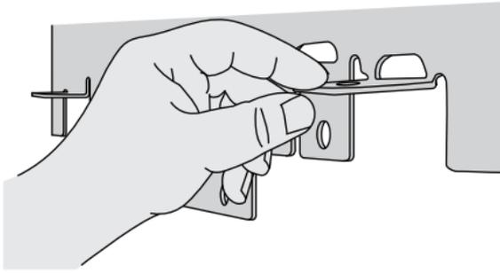
8.) Set FAN into place in the opening using holding tabs, now the tabs hold the fan in position in the ceiling opening.
